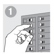
Before beginning **TURN OFF POWER** to the light from fuse or circuit breaker
