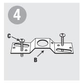
On raised side of offset crossbar (B) thread 1-1/2" mounting screws (C) down through each hole that lines up with canopy.
