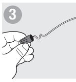
Attach wire nuts to end of each conductor wire.
