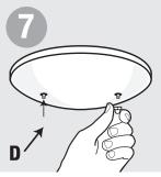
Secure blank-up canopy with cap nuts (D).
