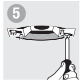
With raised side of crossbar towards ceiling, mount crossbar by inserting 1/2" mounting screws through slotted holes. Tighten until crossbar is flush with ceiling.
